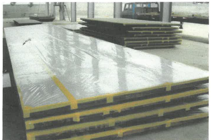
SUS/SS Clad (3+82)x2500 x12000mm
